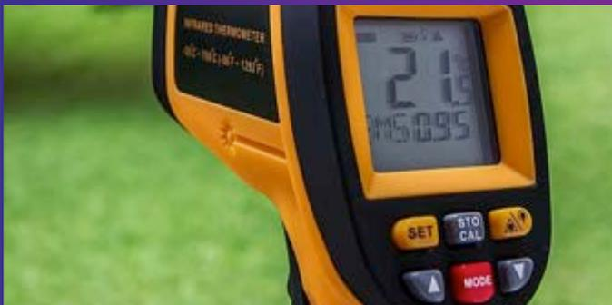
Uses a laser to detect temperatures from a distance. Sometimes accuracy can be affected by surrounding objects. Often used to measure temperatures of moving objects, objects out of reach, or objects too hot or too cold to touch.
