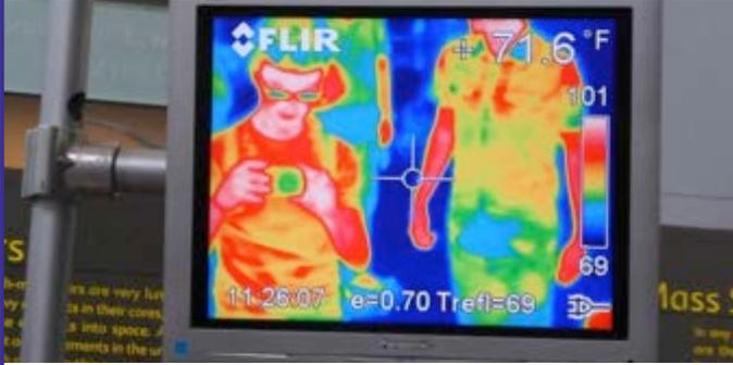
Detects light wavelengths outside the range of human vision and creates an image on a screen. Often used to detect temperature differences. Can also be used for night vision.
