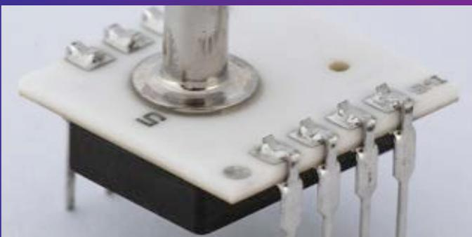
Pressure sensor that detects physical contact. Can sense a squeeze, but cannot measure weight. Often used in everyday objects, such as keyboards, or to test performance of products, like car brakes.
