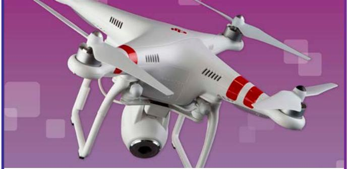
This robotic vehicle flies without a pilot. It is controlled by people on the ground or pre-programmed with missions before take-off. A drone can sense and respond to its surroundings, such as wind, bad weather, or obstacles in its path.
