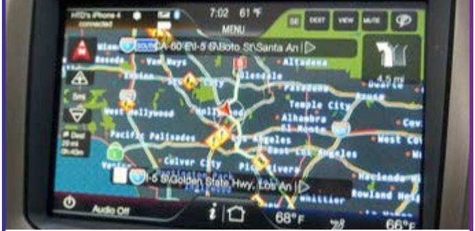
Detects exact location by determining its own distance from satellites orbiting Earth. Often used to track devices and objects, such as in cars and smartphones.
