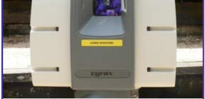
Measures distance, shape and speed of objects by bouncing a laser off an object and analyzing the reflected light. Often used to make high-resolution maps.
